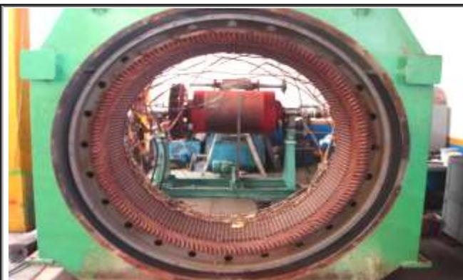
MOTOR SINCRONO DE 2250 HP, MARCA GENERAL ELECTRIC, 4000
